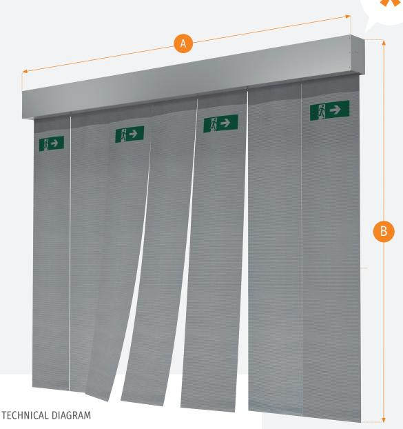
The **TECNITEX MSBEX DH-60/DA-150** smoke controlcurtains are installed in order to fully close off the smoke deposit, lowering to floor level with ASB-3 & ASB-4 systems, their design and configuration in panels allowing the evacuation of people through the system, returning to its functional fire position.
